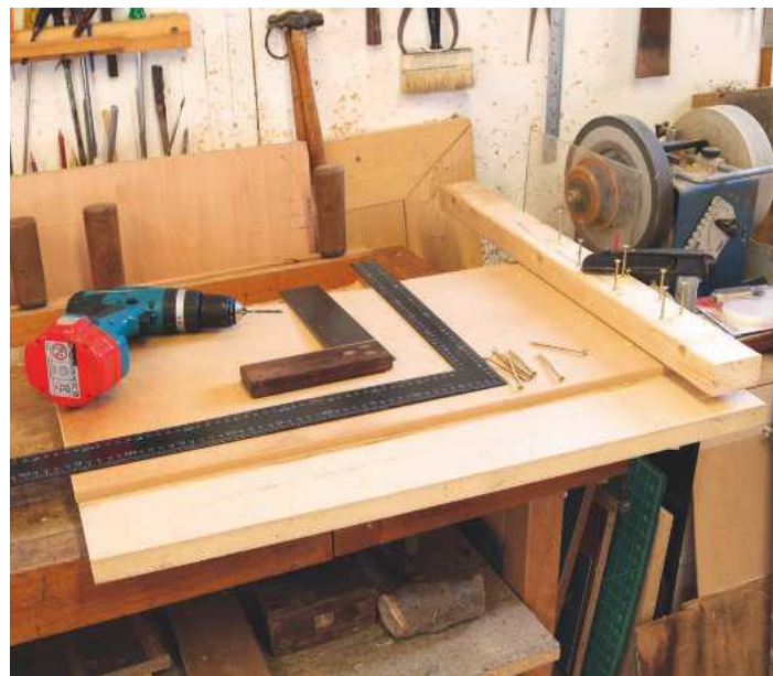
Pic.12 Screw the fence in place with as many screws as will fit
